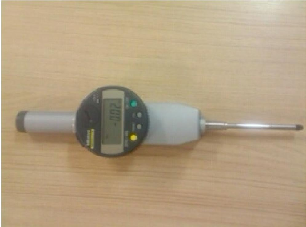
FIGURA 18 – TRANSDUTOR DIGITAL-LVDT
